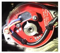
The Rotor / Pickup position as shown is the fully advanced timing position for the system. This is how the parts will align at 3500 RPM and above with the engine running.
