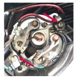
Remove the contact breaker (points) plate by removing the two screws indicated and the condensers. It may be
