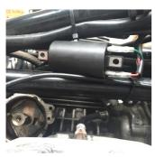
Fit the Tri-Spark dual lead ignition coils (IGC-2006) securely to the frame tube under the fuel tank as shown. Connect the Red and Green wires that were originally going to the distributor points to the ignition coils primary terminals as shown. The wires may be connected either way around as the polarity is not important. There is also a link wire required to connect the 2 coils - see diagram pg 6.
