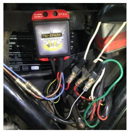
This completes the wiring. Take care to locate the wires away from pinch points, moving parts and hot surfaces.
