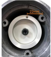
until the FIRST timing mark lines up with the pointer as shown.
