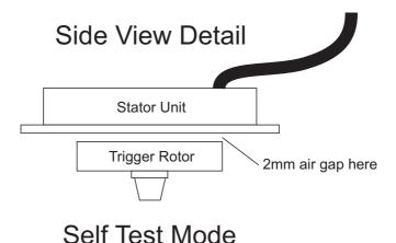
These notes explain how to use the TEST feature on the TRI-0002. By switching on the test mode it is possible to check the operation of the stator unit, rotor, coils, HT leads and spark plugs without starting the engine.
